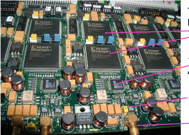
Two FPGAs Per input (400k gates)
